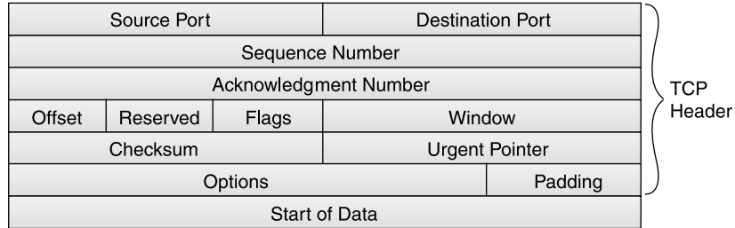
FIGURE 3.2 A datagram with its TCP header
